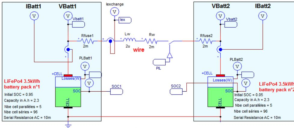
Figure 4 – reference simulations with two batteries in parallel
