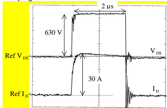
Figure 9 : 500 V MOS waveforms in intrinsic clamping mode
