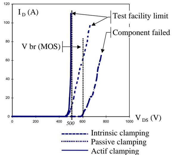
Figure 11 : three dynamics clamping mode characteristics
