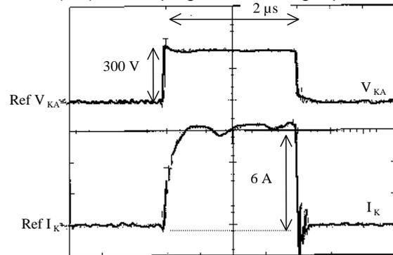
Figure 8 : B2 diode waveforms in clamping mode
