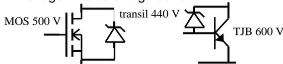
Figure 10 : passive and active clamping examples
