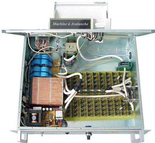
Figure 7 : Avalanche Machine, open
