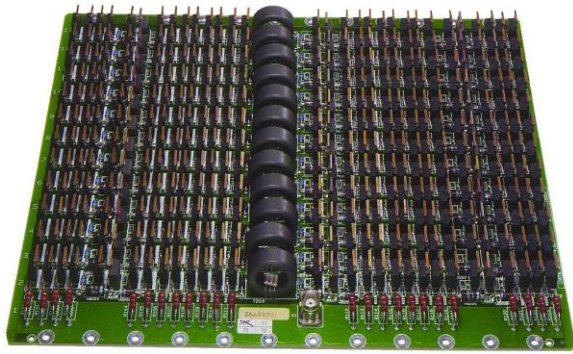
Figure 2 : 350 MOSFETs board switching 5 kV 1000 A CENTRALP
