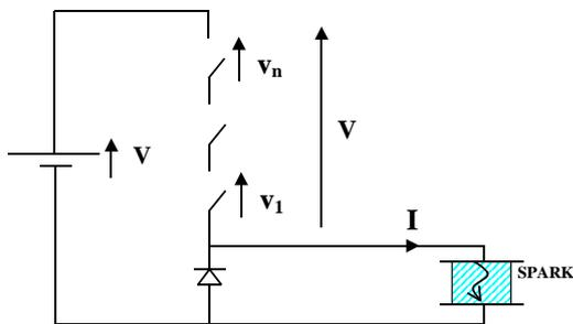
After this current auto-limitation, it's necessary to switch-off the short-circuit current. Because of high  $dI/dt$ , there is an over-voltage generated by stray-inductance. It is necessary to keep all the components in their safety area.
