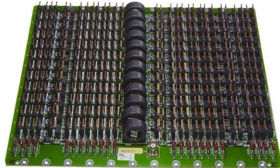
**350 MOSFETs board switching 5 kV - 1000 A
