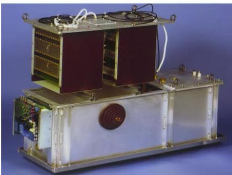
The 1600 A - 25 kV switch is a design of two modules in parallel, each containing five boards in series. Voltage specification for the board is 5 kV. Voltage drop is 20 ns typically.
