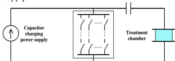
A capacitor or a coaxial line or a pulsed forming network can be used for the energy storage. The thyatron or the matrix mosfet
