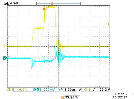
This is the short circuit behavior for a switch. The upper trace is the current in the switch.
