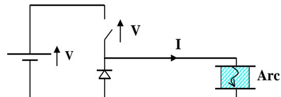
For high voltage fast modulator, the stray inductance has low value, so the short-circuit current is limited by the switch.
