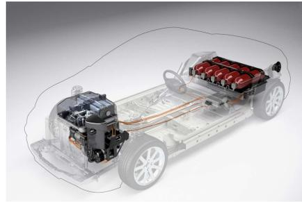
The battery and the hydrogen storage are in the back of the vehicle. The fuel cell system is in the front of the vehicle.
