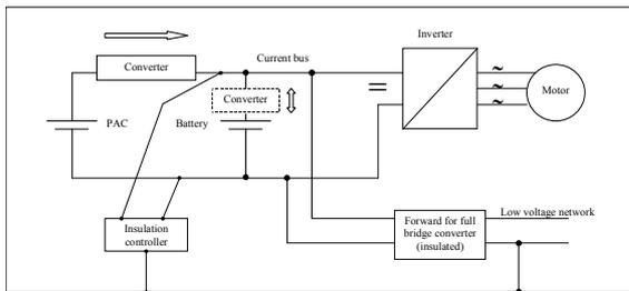
For fuel cell systems of some tens of kilowatts, a boost converter is connected at the output of the fuel cell.
