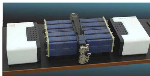
The bipolar plate design is very thin. Bipolar plates and EMA (Electrode Membrane Assembly) are stacked.
