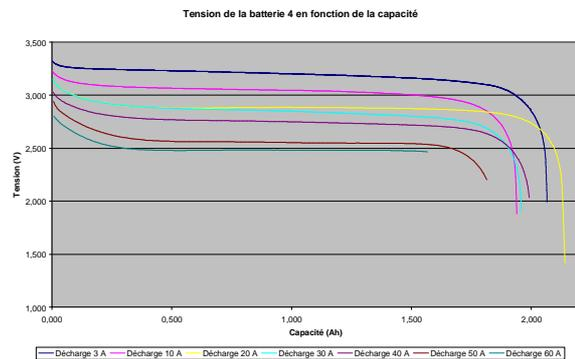
The charge rates are huge for such a standard accumulator. The different curves are for the following discharge rates.
