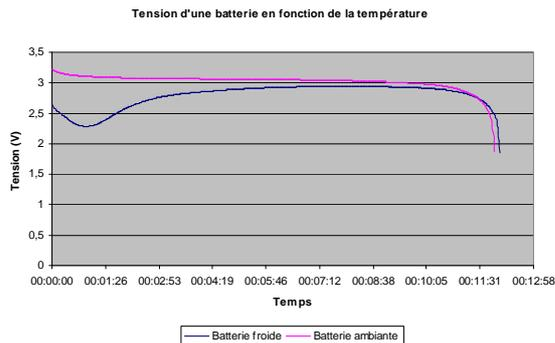
Because of the higher internal resistance, losses are more important. There is a temperature rise. At higher temperature, the internal resistance decrease and the voltage drop decrease too.
