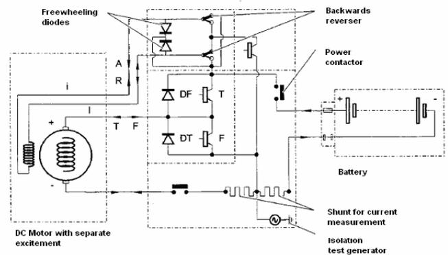
Figure 6: synoptic diagram of the converter
