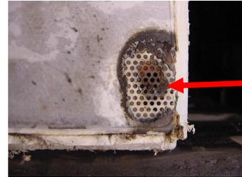
Figure 10: degradation of the separators, follow-up of fusion.
