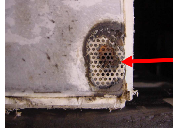
Fig. 5. : Degradation of the separators, follow-up of fusion.
