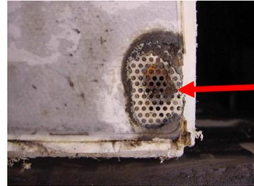
**Fig. 5.** : Degradation of the separators, follow-up of fusion.
