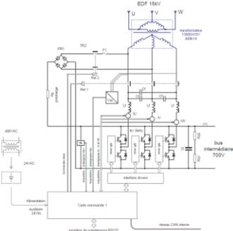
An inverter absorbs sinusoidal current on the three phases to generate a 700 V intermediary bus.
