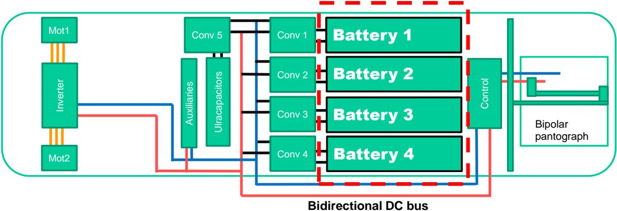
Figure 2: bus electrical architecture
