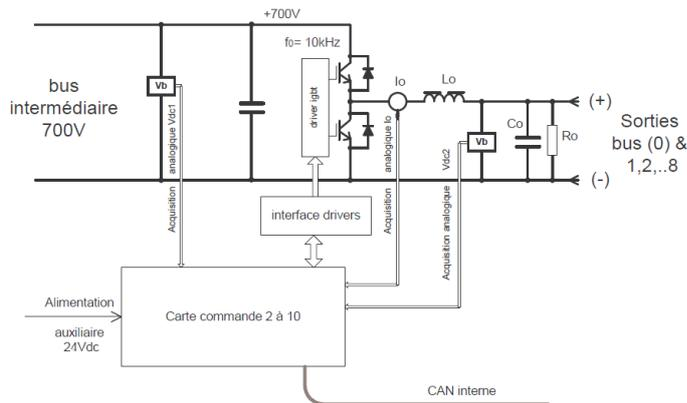
Bidirectional buck converters are used to provide a constant voltage output to supply the bus.
