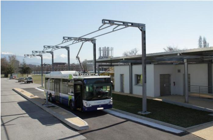
Figure 8: CEA 350kW charge station
