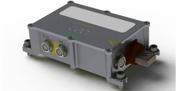
Figure 7: BMS central microcontroller
