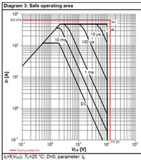
**Fig.14:** Device n°1 safe operating area during avalanche
