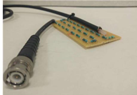
**Fig.12:** Handmade 5kΩ probe
