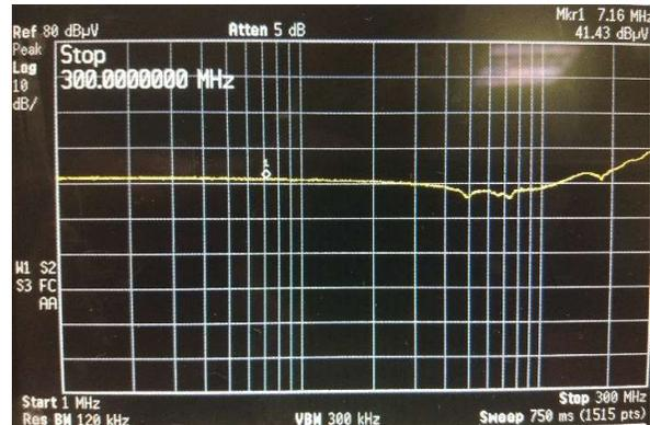
**Fig.13:** Bandwidth of the 5kΩ probe
