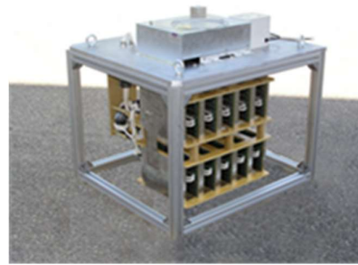
Fig. 7: 100 kV 25 A Turn on, turn off and short circuit proof switch for Tore Supra.
