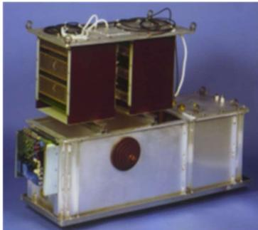
**Fig. 1:** 25 kV 2000 A switch for two thyatrons replacement
