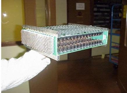
**Fig. 5:** 10 kV 500A Turn on, turn off and short circuit proof switch, diodes side
