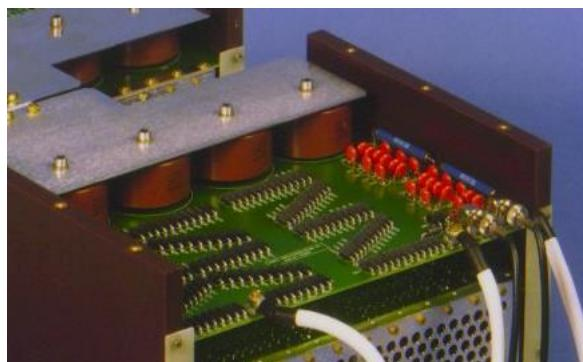
On the right part of the photograph is the high voltage probe with two high voltage resistors and small standard capacitors in series. It's a low cost solution for voltage measurement.
