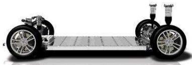
Figure 6: TESLA model S battery concept
