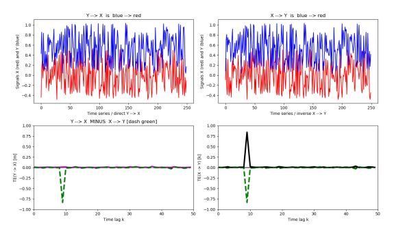
Figure 1. (Top left and right) Time traces of the two processes X and Y over which TE is computed. For visualisation purposes only, Y is offset by its maximum value. TE  $(Y \rightarrow X)$  is represented (lower left) in purple and TE  $(X \rightarrow Y)$  in black (lower right) as a function of time lag k. The net Transfer Entropy  $\Delta_{X,Y}$ (TE) is displayed as well (dashed green).
