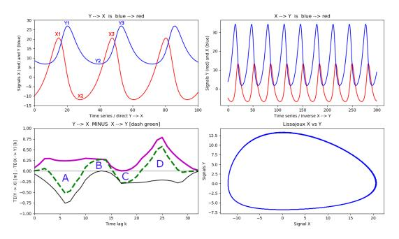
This illustrates causality in the flow of time and clarifies the reason of  $TE(X \rightarrow Y)$  peaking at time lags = 29, 91, ... (bottom right panel). It also shows that the TE technique does not require many occurrences of causal events to unambiguously extract relevant flows of information.
