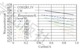
Figure 11: Example of current tunability at fixed temperature of our QCL ship
