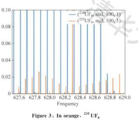
rotational lines are inside the rotational structure of  $^{238}$  UF<sub>6</sub> , in blue
