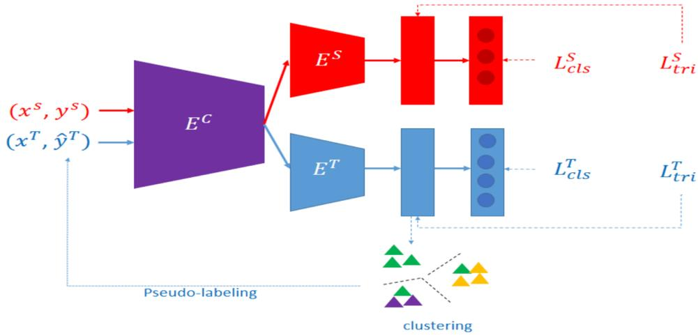
Fig. 1. Unlike existing pseudo-labeling strategies (1), our framework is a source-guided (3) as it leverages the labeled source dataset during pseudo-label training. It is composed of a shared encoder  $E^C$  and two domain-specific branches  $E^S$  and  $E^T$ . The numbers of shared layers and specific layers can vary. Configuration (2) represents the extreme case when all layers are shared and there is no domain-specific branch.
