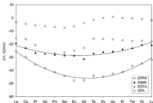
**Fig. 7** Variation of  $\Delta H^\circ$  across the lanthanide series for the complexation of Ln(III) with NTA, DTPA, EDTA in aqueous solution<sup>22</sup> and Adptz in MeOH–H<sub>2</sub>O solution (76%/24% vol).
