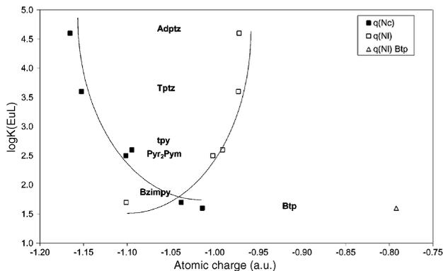
**Fig. 3** Correlation between the atomic charges on N<sub>l</sub> and N<sub>c</sub> in [EuL]<sup>3+</sup> complexes calculated in the gas phase and the stability constants of [EuLA<sub>3</sub>] complexes (A = Cl<sup>-</sup>, ClO<sub>4</sub><sup>-</sup>) in MeOH–H<sub>2</sub>O solution (room temperature).
