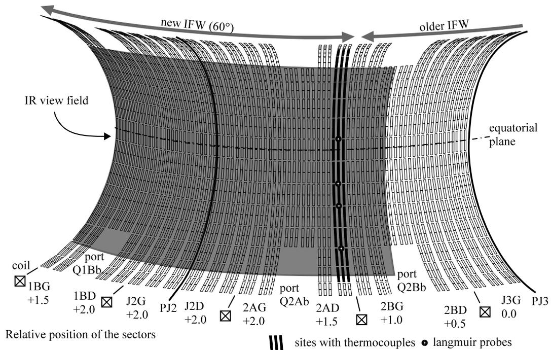
**figure 1 : diagnostics of the Inner First Wall**
