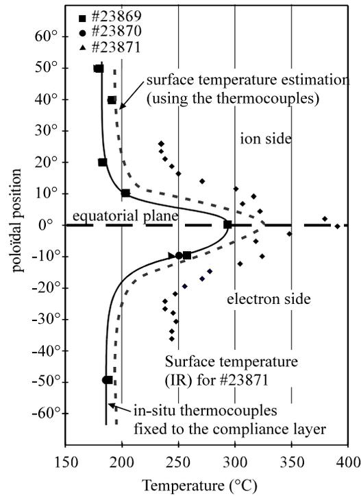
**figure 3 : Poloidal profile of the temperature**
