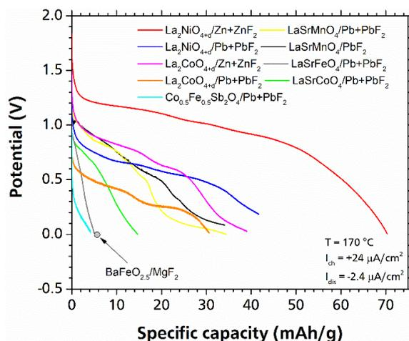
Figure 21. Discharge profiles of some of the so far proposed intercalation-based cathode materials for FIBs. Reproduced with some modifications from ref.<sup>27</sup>.
