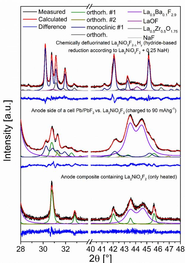
Figure 22: Comparison of selected angular ranges of XRD patterns of chemically (top) and electrochemically (middle) defluorinated  $\text{La}_2\text{NiO}_3\text{F}_{2-x}$ . The chemical defluorination was obtained via a hydride-based reduction, the electrochemical
