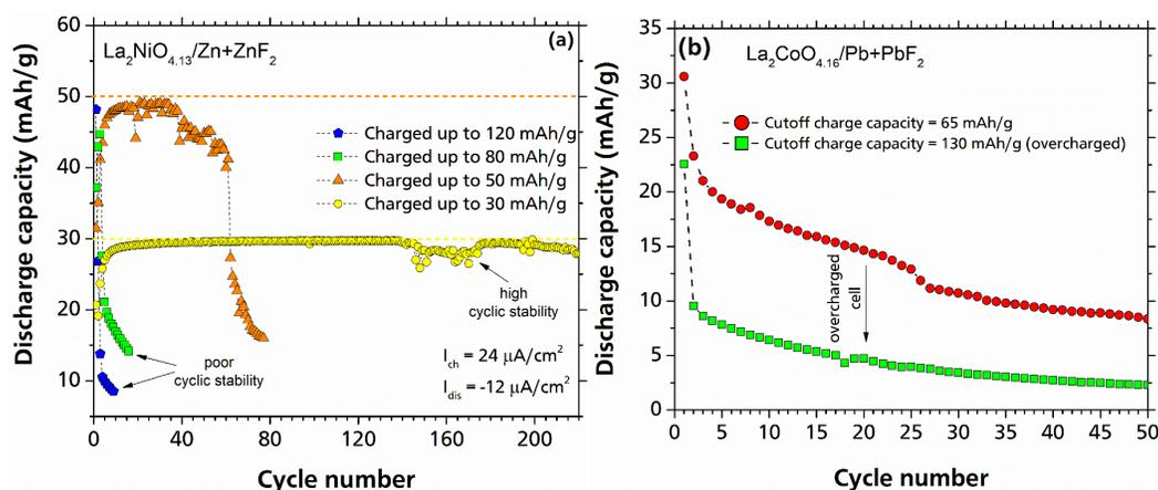
Figure 17. (a) Cycling stability of the  $\text{La}_2\text{NiO}_{4.13}|\text{Zn}+\text{ZnF}_2$  cell at different cutoff capacities<sup>151</sup>; (b) the effect of overcharging on cycling stability of a  $\text{La}_2\text{CoO}_{4.16}|\text{Pb}+\text{PbF}_2$  cell. All cells were heated at 170 °C and charged/discharged at a current of 24/-12  $\mu\text{A}/\text{cm}^2$ . Reproduced from ref.<sup>29</sup>.
