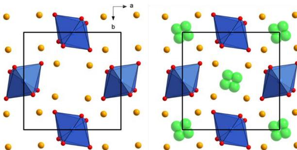
Figure 20. Schematic presentation of the non-fluorinated  $MSb_2O_4$  (left) and fluorinated  $MSb_2O_4F_y$  (right) Schafarzikite-type structure. Sb orange, M (Fe, Co) blue, O red, F (partially occupied to ~15 %) green. Reproduced from ref.<sup>158</sup> (open source publication).
