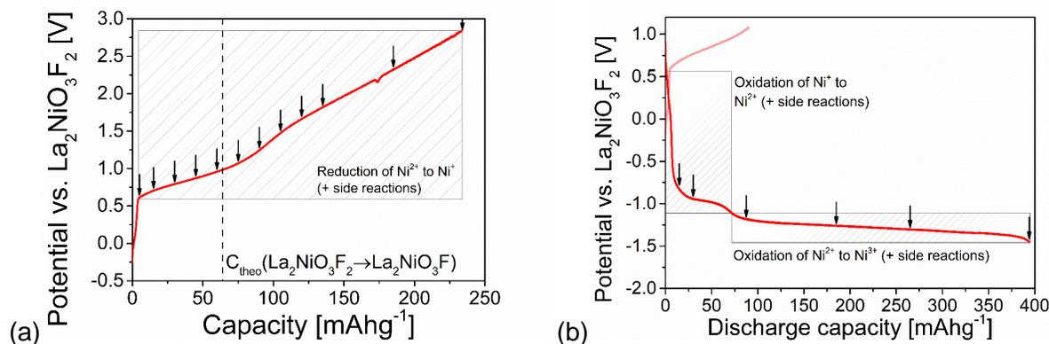
Figure 23: a) Charging curve of a cell  $\text{Pb}+\text{PbF}_2$  against  $\text{La}_2\text{NiO}_3\text{F}_2$ , b) Charging and discharging curves of a cell  $\text{Pb}+\text{PbF}_2$  against  $\text{La}_2\text{NiO}_3\text{F}_2$ . The cell was charged to  $90 \text{ mAh g}^{-1}$  prior to the discharging. The cells were heated to  $170 \text{ }^\circ\text{C}$ , a current of  $\sim 2.5 \text{ mA g}^{-1}$  ( $\sim C/25$  rate) was applied. Reproduced from ref.<sup>34</sup>.
