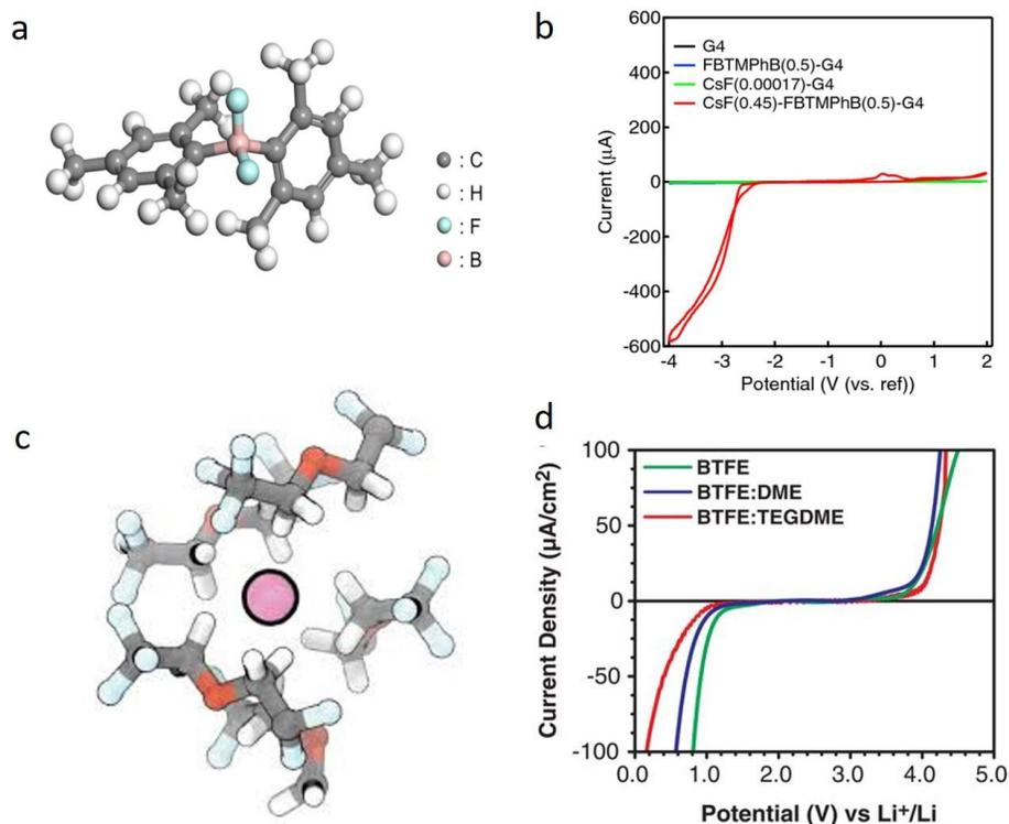
Figure 12. (a) Optimized molecular structure of FBTMPbB-F<sup>-</sup>, (b) Cyclic voltammograms of the CsF(0.45)-FBTMPbB(0.5)-G4 (parts a and b are reproduced from ref.<sup>110</sup> with permission<sup>xii</sup>); (c) Simulated solvation shell of BTFE molecules surrounding F<sup>-</sup> (pink sphere) (d) Linear sweep voltammograms for 0.75 M Np1F in BTFE, collected using a scan rate of 1 mV.s<sup>-1</sup>. (parts c and d are reproduced from ref.<sup>33</sup> with permission<sup>xiii</sup>)
