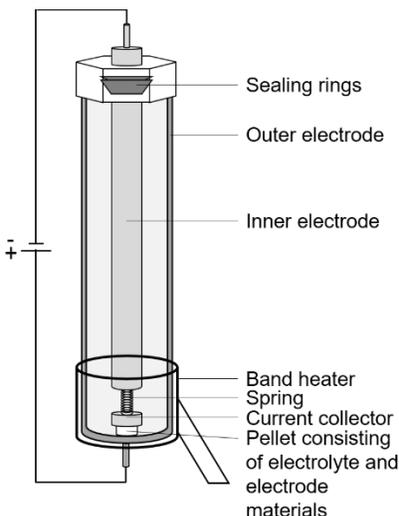
Figure 3. A schematic of a high-temperature cell used for the electrochemical measurements conducted on all-solid-state FIBs. The figure has been reproduced from ref. <sup>34</sup>.
