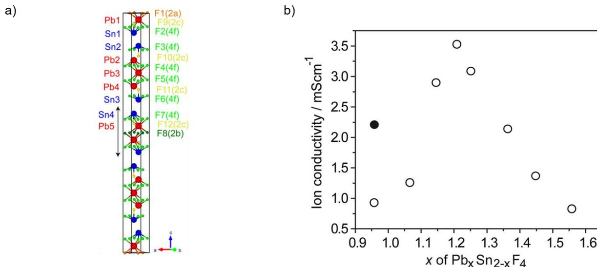
Figure 10. (a) Packing of  $\beta^+\text{-PbSnF}_4$  in the unit cell. Blue and red balls are Sn and Pb, respectively. (b) Dependence of the conductivity at room temperature on the Pb/Sn molar ratio in the  $\text{Pb}_x\text{Sn}_{2-x}\text{F}_4$  pressed-powder samples ( $x = 0.96\text{--}1.56$ ) annealed at 400 °C (open circle) and 200 °C (filled circle) (figures are reproduced from ref.<sup>74</sup> with permission\*).
