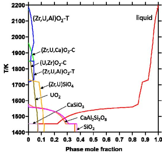
Figure 10 : Calculated solidification path of liquid#1 phase
