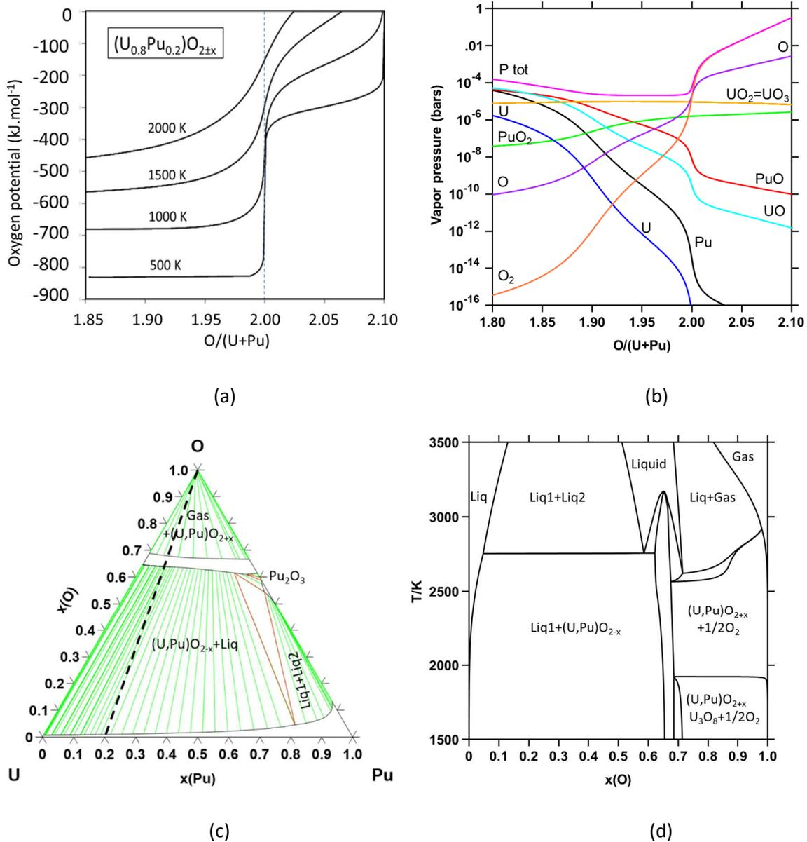
Figure 4: Calculated (a) oxygen potential of  $(U_{0.8}Pu_{0.2})O_{2\pm x}$  as function of  $O/(U+Pu)$  ratio at 500, 1000, 1500 and 2000 K ; (b) vapor pressure of the gaseous species and total pressure above  $(U_{0.8}Pu_{0.2})O_{2\pm x}$  as function of  $O/(U+Pu)$  at 2300 K ; (c) isothermal section of the U-Pu-O system at 2300 K ; (d) isopleth section of the U-Pu-O system with  $U/Pu=4$  along the composition line reported on the isothermal section (dashed line).
