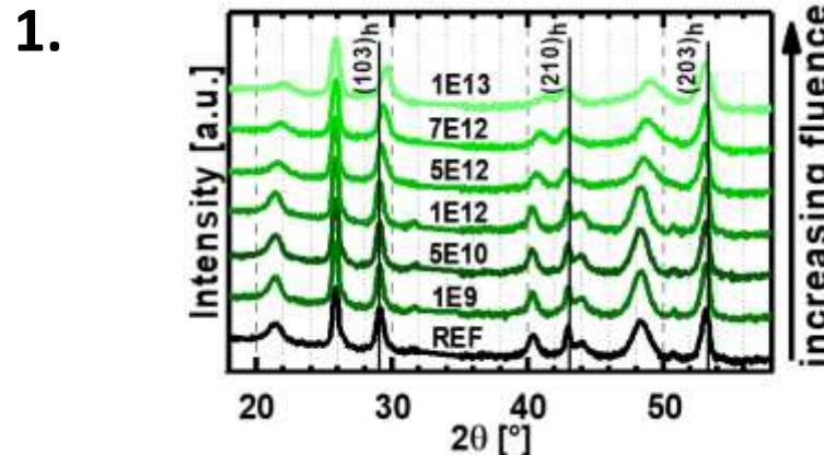
Fig. 6 XRD patterns of GST crystalline layers before (REF) and after irradiations at increasing fluence.
