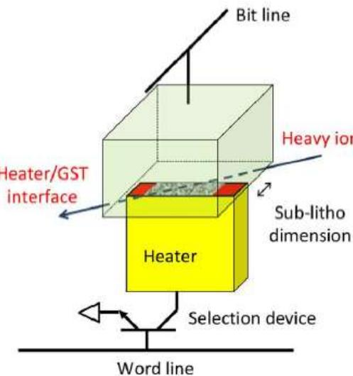
Fig. 4 Schematic of a phase change memory device hit by a heavy ion along the word line [4].
