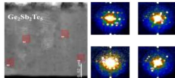
Fig. 7 TEM (left) and nano-diffraction patterns (right) analyses of as-deposited amorphous GST after irradiation at a fluence of  $10^{13}$  ions/cm<sup>2</sup>.
