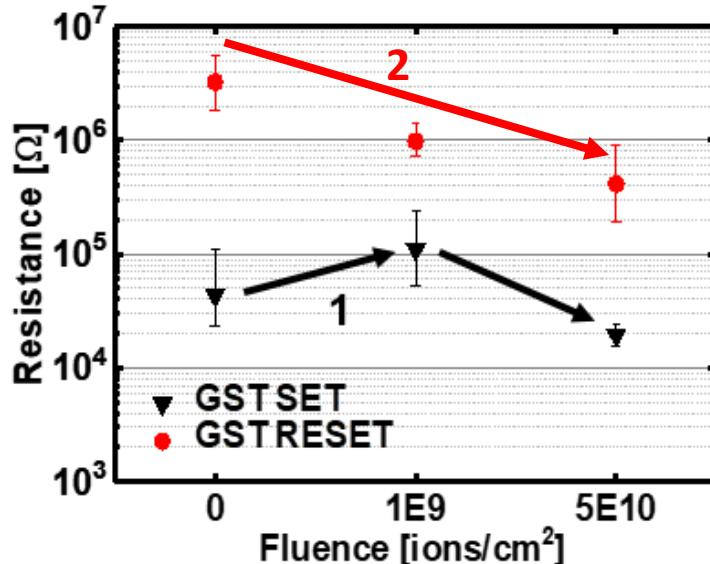
Fig. 5 Median and  $\pm\sigma$  for SET and RESET distributions in GST 4kb arrays before and after irradiations at increasing fluences.
