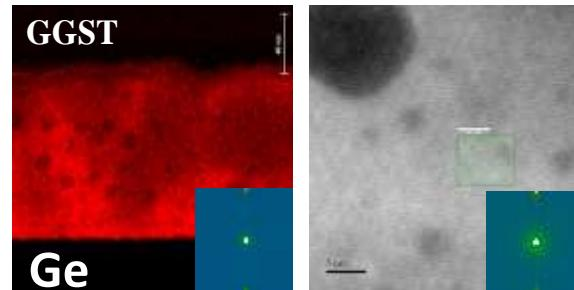
Fig 12 TEM/EDX and nano-diffraction patterns analyses of crystalline GGST after irradiation at a fluence of  $7 \times 10^{12}$  ions/cm². The Ge cartography (left) shows that the Ge segregation induced by the annealing process remains unchanged after irradiation. However, the irradiation reduces the size of the crystallites as evidenced by few and low intensity nano-diffraction patterns identified (right).
