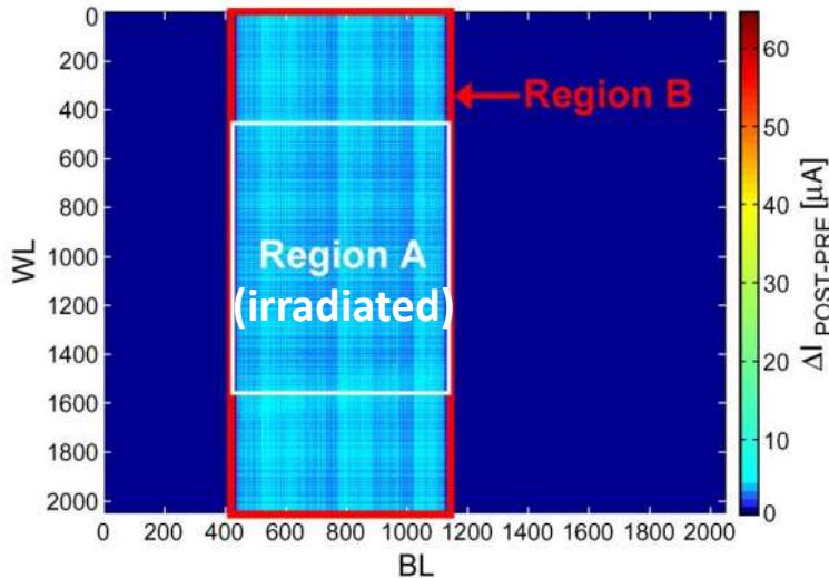
Fig. 3 Color map of the value of the cells of a MOS-chip array irradiated with a 30 Mrad SiO<sub>2</sub> proton beam. Region A is the irradiated zone and Region B is the area where the cells show a change in current of more than 1 A with respect to the pre-irradiation condition [3].
