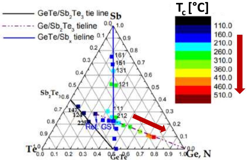
Fig.2 Crystallization temperatures  $T_c$  as a function of compositions in the Ge-Sb-Te ternary phase diagram [2]
