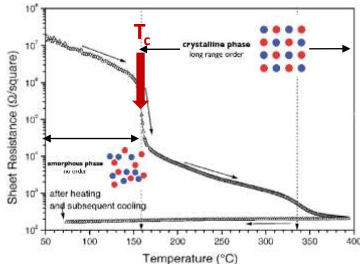
Fig.1 Resistivity as a function of temperature of a Phase-Change Material [1]
