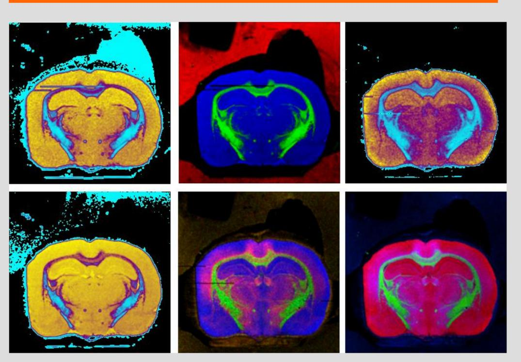
Examples of images from secondary ions mass spectrometry (TOF-SIMS) of different lipids (choline, phosphocholine, phospholipids, fatty acid, cholesterol, vitamin E) on the surface of a rat brain sample. Images sizes: 18x18 mm², 256x256 pixels of 70x70 µm².
