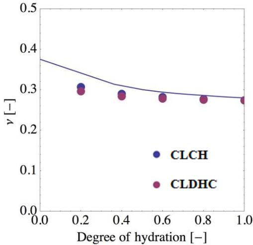
Figure 7. Poisson ratio of concrete: Numerical (dots) and MT (line)
