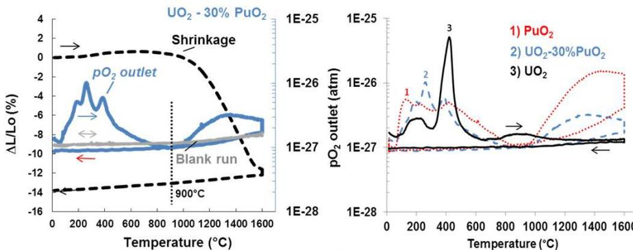
By integrating the overall oxygen loss measured throughout the experiment we can calculate the corresponding weight loss. Considering that each material O/M ratio is equal to 2.00 at 900°C, it is possible to derive the evolution of the O/M ratio.
