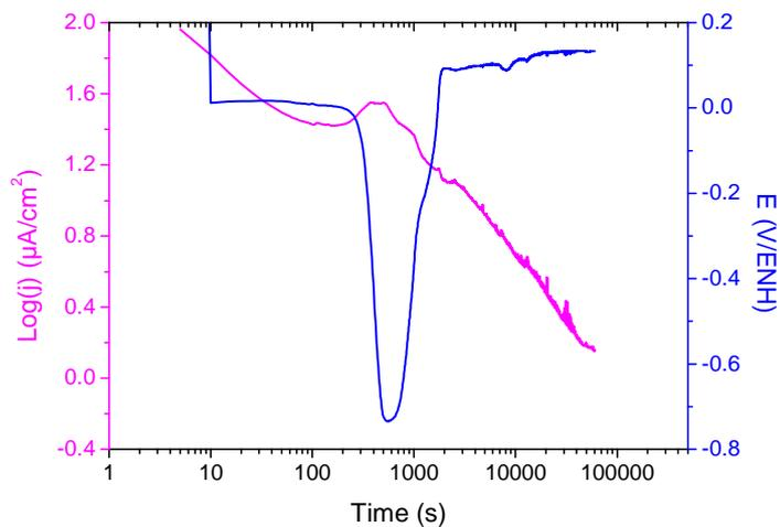
**Figure 6:** Potential and galvanic density current values as a function of time for Mg alloy coupled with Pt, in ZRA mode without stabilization in 0.1M NaOH.
