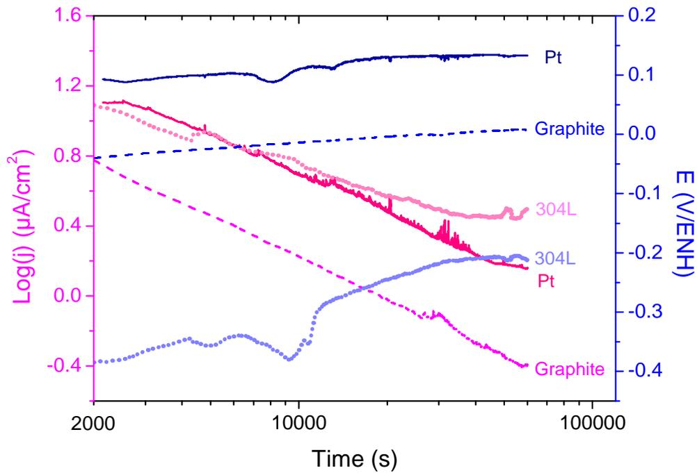
**Figure 7:** Potential and galvanic density current values as a function of time for Mg alloy coupled with Pt, graphite or 304L in ZRA mode after transient regime.
