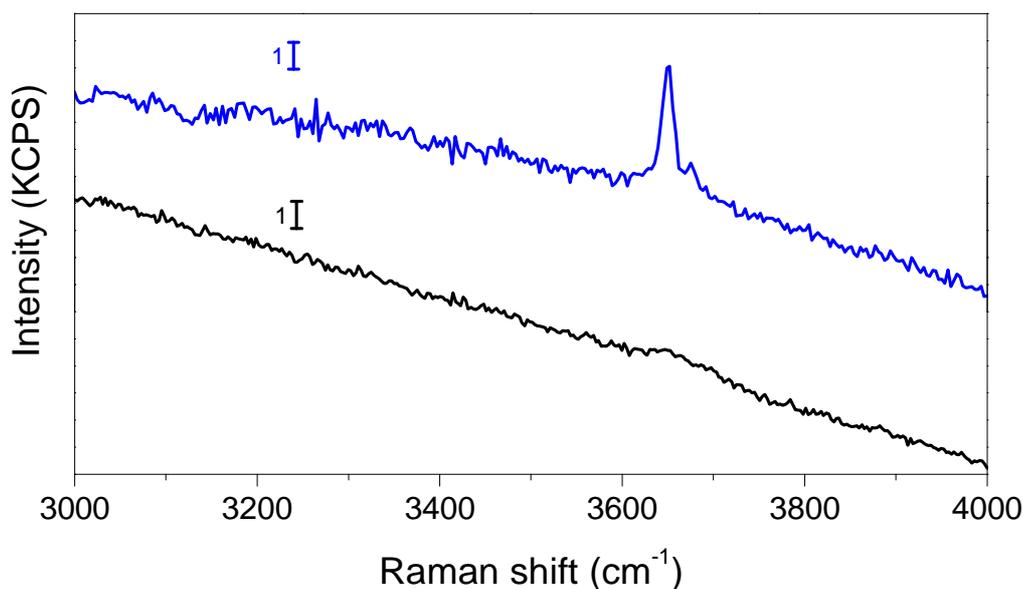
**Figure 9:** Raman spectra of Mg alloy before (in black) and after (in blue) galvanic coupling with Pt during 16h in 0.1M NaOH.
