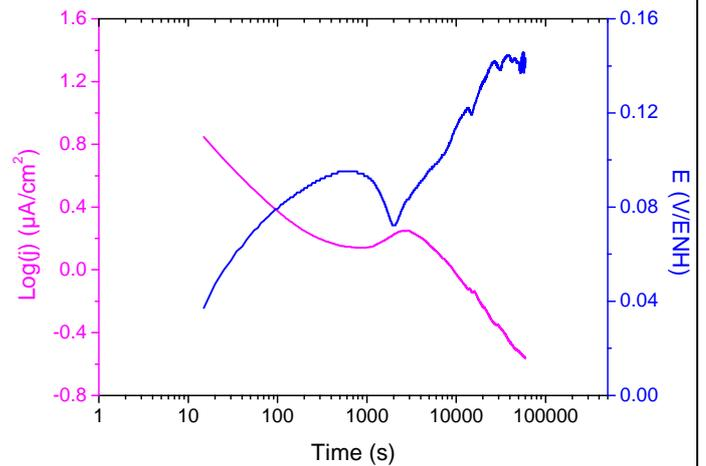
**Figure 5:** Potential and galvanic density current values as a function of time for Mg alloy coupled with Pt, in ZRA mode after 1h of stabilization in 0.1M NaOH.
