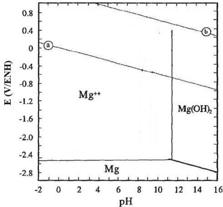
**Figure 1:** E-pH diagram of Mg in aqueous solution at 25 °C. The lines a and b identify the reaction of hydrogen and oxygen evolution, respectively [7].
