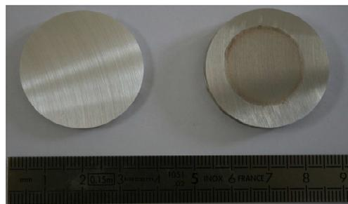
**Figure 8:** Mg alloy sample before (on the left) and after (on the right) galvanic coupling with graphite during 16h in 0.1M NaOH.
