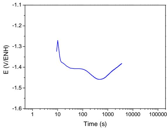
**Figure 4:** Potential values of Mg alloy as a function of time in 0.1M NaOH.
