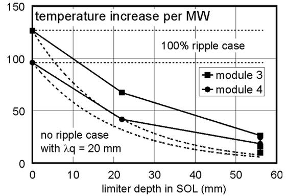
**Figure 5 :** Maximum surface temperature increase per MW of ICRH, as a function of the distance between the limiter and the LCFS. The two pairs of dashed lines are the theoretical cases of surface temperature increase with 0 and 100% ripple losses. Data are plotted for two areas in modules 3 and 4 (modules are 60° toroidal sections of the TPL).
