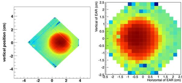
**Figure 5.** Neutron beam images obtained using a MicroMegas detector with XY strips (left panel). and with a pixellized MicroMegas. Figures are from ref. [18].
