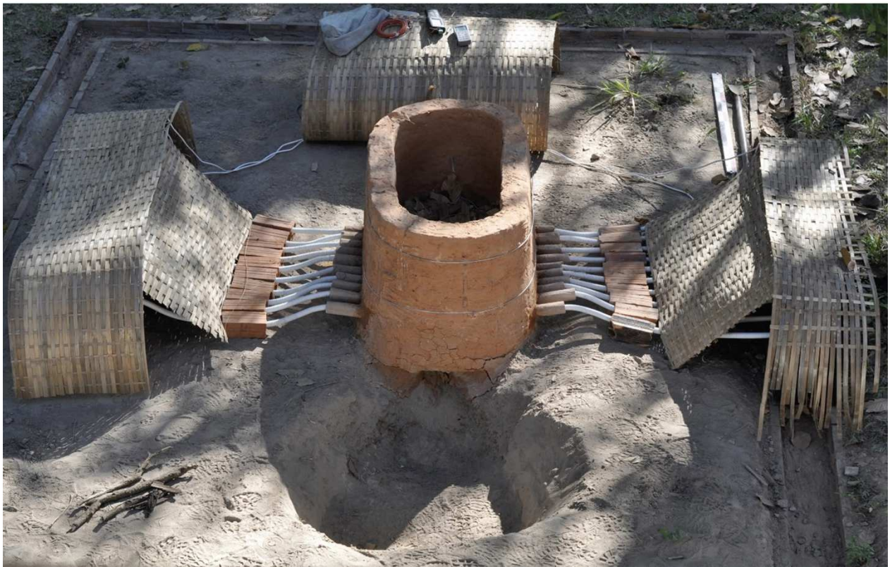
Figure 5: Schematic proposition and final construction of the experimental furnace and air supply system.
