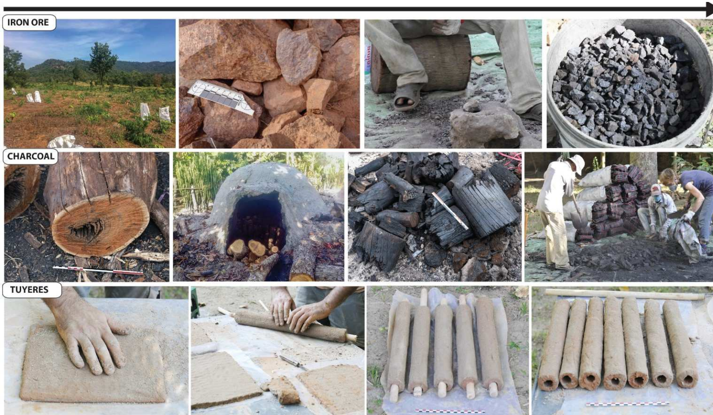
Figure 6: The different stages of preparation for the ore, charcoal and tuyères.
