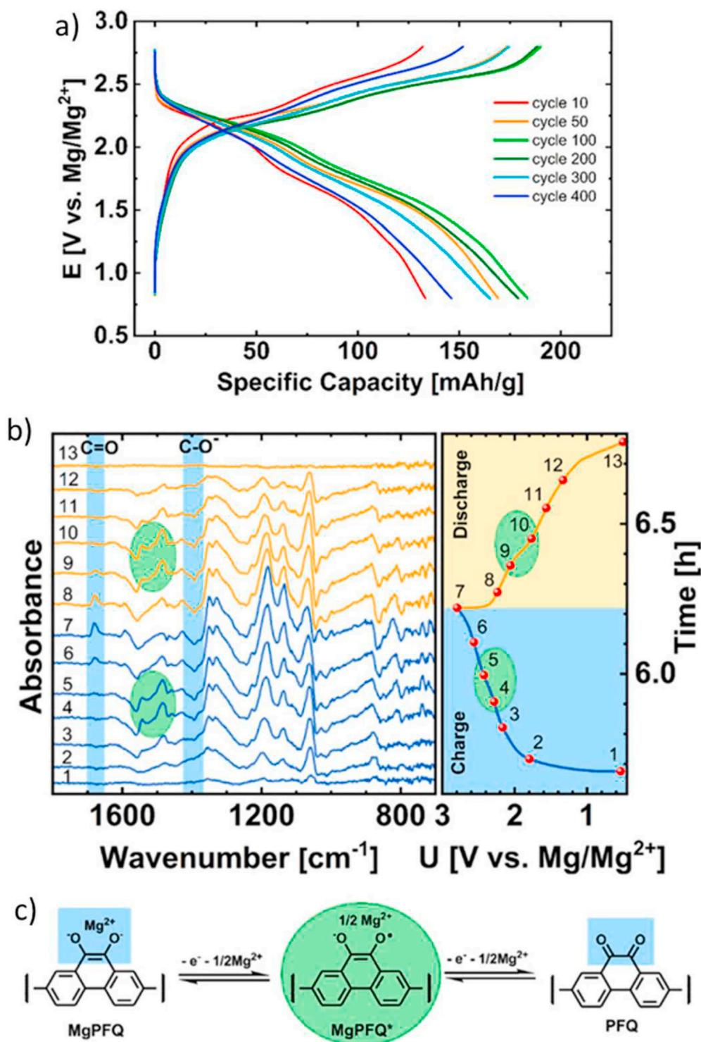
Fig. 8. Electrochemical cycling and electrochemical mechanism of poly(phenanthrene quinone)/reduced graphene oxide cathode (PFQ/rGO). a) Long-term cycling of PFQ/rGO at 0.5C in  $Mg(TFSI)_2$ - $2MgCl_2$  in DME electrolyte. b) Subtracted *operando* ATR-IR spectra of organic cathode displaying IR active changes during electrochemical cycle. c) Proposed electrochemical mechanism of PFQ/rGO cathode. Reproduced from reference 148 under open access CC BY 4.0 license.
