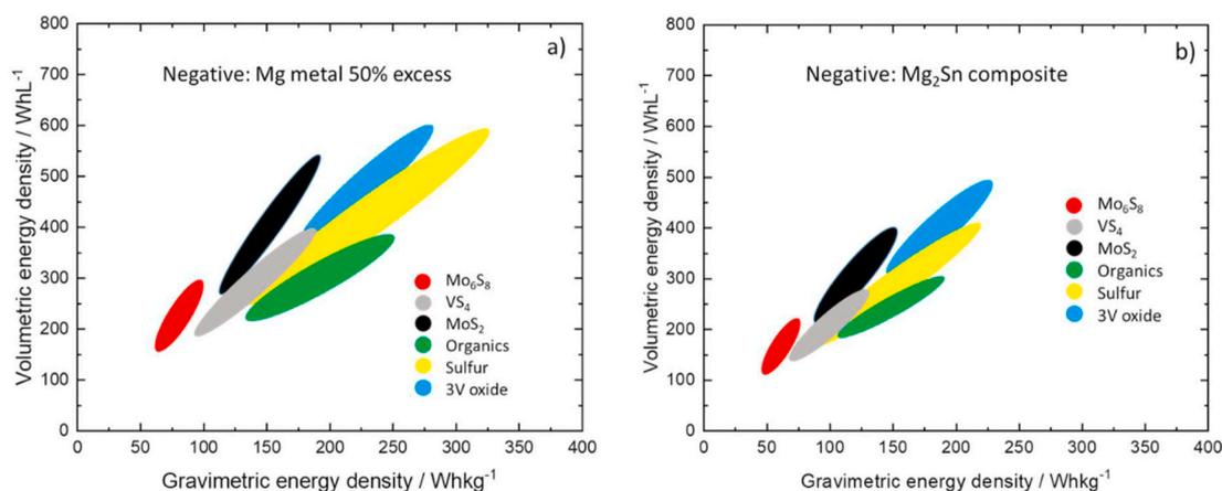
Fig. 1. Correlation maps between volumetric and gravimetric energy densities of different cathodes operating under two different anodic scenarios: a) pure magnesium metal with 50 wt% excess and b)  $\text{Mg}_2\text{Sn}$  alloy. Figures were derived from calculations presented in Figs. S1 and S2.
