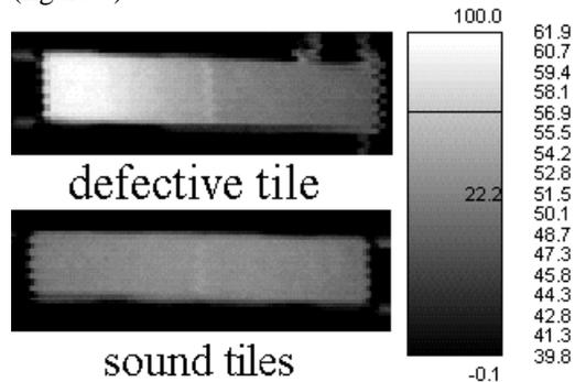
**Figure 7 : Defect on a PPI element**
