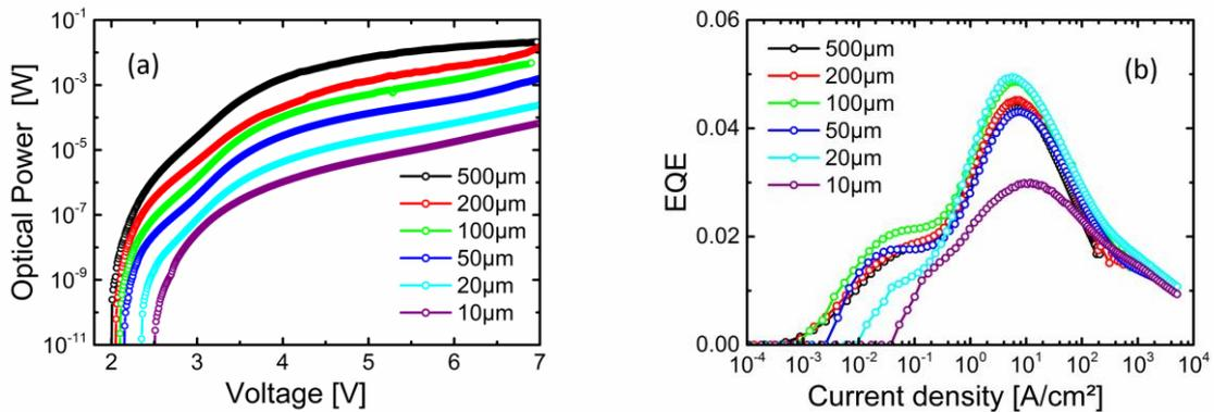
Figure 2. (a) Optical power versus voltage and (b) external quantum efficiency versus current density characteristics of different square  $\mu$ LEDs. Two different optical regimes are depicted on large scale  $\mu$ LEDs. The 1<sup>st</sup> regime tends to disappear for smaller  $\mu$ LEDs. It is worth noting that the 1<sup>st</sup> regime vanishing is correlated to the shift of the optical emission threshold also observed on smaller geometry  $\mu$ LEDs.
