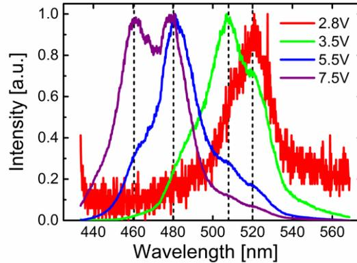
Figure 7. Normalized electroluminescence spectra versus bias carried out on a  $6\mu\text{m}$  diameter  $\mu$ LED. In contrary to what is usually believed, the blue shift in InGaN/GaN  $\mu$ LEDs is not solely due to the QCSE. The appearance of discrete emission peaks with variable intensities depending on injection bias level tends to corroborate the filling of high excited levels in the quantum wells explaining the color changing behavior in green  $\mu$ LEDs.
