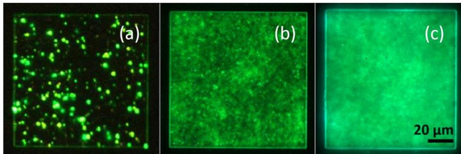
Figure 4. Optical photos of light emission homogeneity on a  $100 \times 100 \mu\text{m}^2$  green LED at different bias values: (a)  $V = 2.2\text{V}$ , (b)  $V = 3.5\text{V}$  and (c)  $V = 4.5\text{V}$ . Note the high luminance spread at low voltage that disappears at higher bias values.
