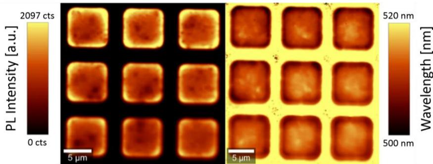
Figure 3. Photoluminescence intensity and wavelength mappings on a  $3 \times 3$   $7 \mu\text{m}$  squared  $\mu$ LEDs array. A higher intensity correlated to a shorter wavelength emission is observed on the edges of  $\mu$ LEDs. We suppose a probable lattice relaxation at the edges of  $\mu$ LEDs, reducing the QCSE effect behind this observation.
