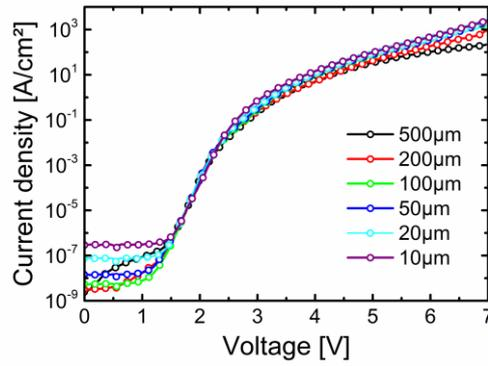
Figure 1. Current density versus voltage characteristics of different square  $\mu$ LEDs. Current density is constant on a large bias range whatever the  $\mu$ LED size is. The legend denotes the side width of each  $\mu$ LED.
