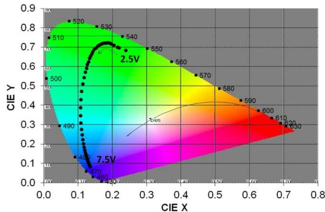
Figure 6. Color point evolution of the emitted light from a green  $\mu$ LED plotted on CIE chromaticity 1931 diagram. Bias varies from 2.5V to 7.5V. Each point corresponds to 100mV increase in voltage. The measured wavelength varies from 540nm (green) to 475nm (blue).
