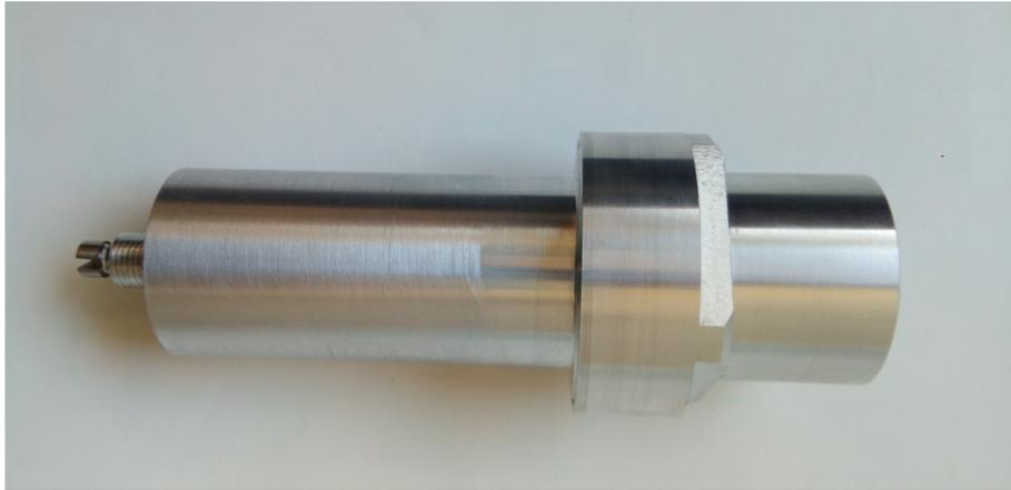
Figure 1: CANOE mock-up. of CANOE. The neutron sensitive layer is enriched a boron carbide, coupled with a 200  $\mu\text{m}$ -diameter core silica fiber, with no use of focusing assembly.
