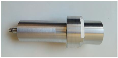
Figure 1: CANOE mock-up. of CANOE. The neutron sensitive layer is enriched a boron carbide, coupled with a 200  $\mu m$ -diameter core silica fiber, with no use of focusing assembly.
