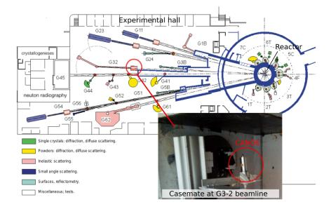
Figure 3: Experimental setup at ORPHEE. The G3-2 cold neutron beamline of a  $25x50 \text{ mm}^2$  section provides a mono-directional flux as low as 8E8 n.cm<sup>-2</sup>.s<sup>-1</sup>.
