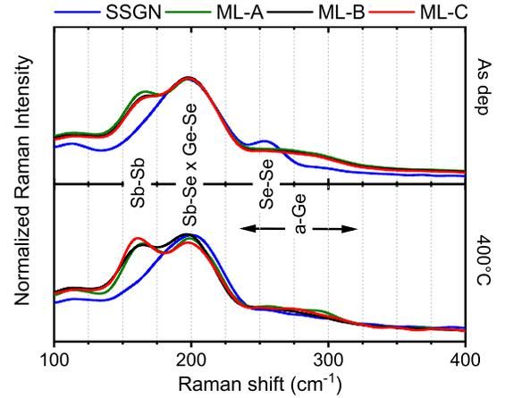
**Fig. 4.** Raman spectra for SSGN and MLs as deposited (top) and after 400°C annealing (bottom). All spectra are normalized using the main feature at 200  $\text{cm}^{-1}$  that results from correlation of  $[\text{SbSe}_{3/2}]$  and  $[\text{GeSe}_{4/2}]$  features. Homopolar Sb-Sb bonds are part of the more complex feature  $(\text{Se}_2)\text{Sb}(\text{Ge})\text{-Sb}(\text{Se}_2)$  [10], [11] that stabilizes after annealing.
