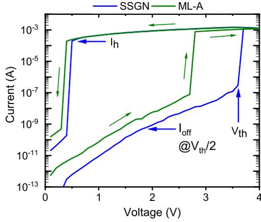
**Fig. 5.** Quasi-static curves for SSGN and ML-A, demonstrating the compatibility of the switching behavior between OTS ML and bulk OTS. We define the leakage current ( $I_{\text{off}}$ ), measured at  $V_{\text{th}}/2$ , and the holding current ( $I_h$ ).
