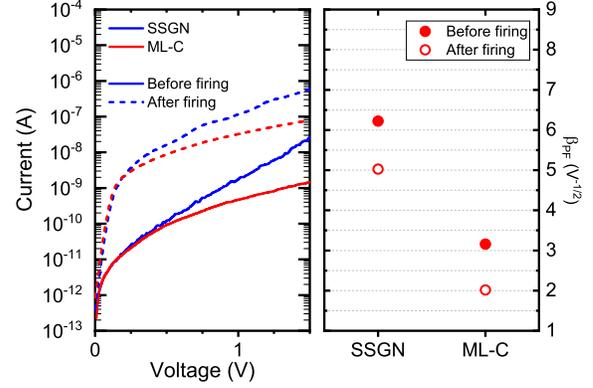
Fig. 11. Subthreshold IV curves before and after firing for SSGN and ML-C after the  $400^\circ\text{C}/30\text{min}$  annealing (only median curves are shown) (left) and correspondent subthreshold conductivity slope  $\beta_{PF}$  (right).
