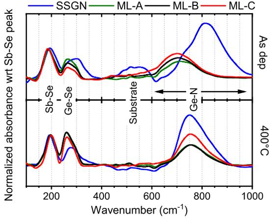
**Fig. 2.** FTIR spectra of SSGN and MLs (top) as deposited and (bottom) after a 400°C annealing. The peak at 266  $\text{cm}^{-1}$  corresponds to  $\text{GeSe}_4$  ( $\nu_3$  mode) which is privileged in multilayer structure while the shoulder at 300  $\text{cm}^{-1}$  should correspond to  $\text{GeSeGe}$  ( $\nu_1$  mode) [6], [7] that is more intense in bulk SSGN. After annealing, SSGN bond network evolves to a structure comparable to MLs.
