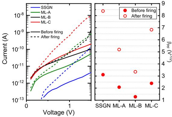
**Fig. 6.** Subthreshold IV characteristics before and after firing for SSGN and MLs (only median curves are shown) (left). Subthreshold conductivity slope  $\beta_{PF}$  is calculated for all the samples (right).
