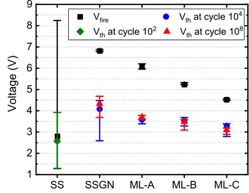
**Fig. 7.**  $V_{\text{fire}}$  and  $V_{\text{th}}$  after  $10^4$  and  $10^8$  cycles for SSGN and MLs. SSGN shows higher  $V_{\text{fire}}$  and  $V_{\text{th}}$  values and higher variability wrt MLs. SS parameters are shown only up to  $10^2$  cycles since after the material triggers crystallization.
