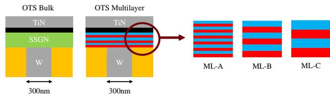
Fig. 1. Simplified description of our OTS ML device compared to standard OTS. The bottom electrode consists in a tungsten plug with a diameter of  $\sim 300$  nm. A carbon intermediate electrode is fabricated between the top electrode and the OTS material to prevent intermixing among the two during cycling operations.
