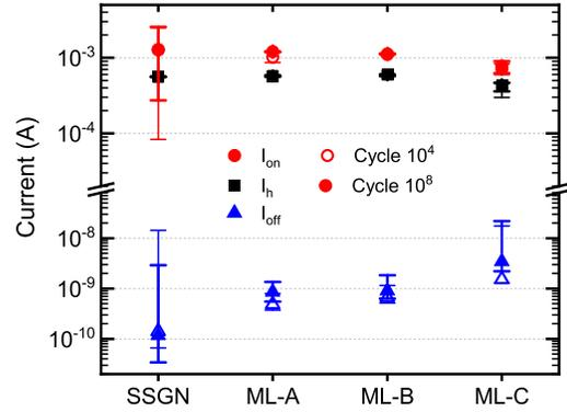
**Fig. 8.** Electrical parameters  $I_{\text{on}}$ ,  $I_h$  and  $I_{\text{off}}$  after  $10^4$  and  $10^8$  cycles for SSGN and MLs. Identical results are achieved with both RESET and SET-like pulses conventionally used for Phase-Change Memory applications (not reported for graph clarity).
