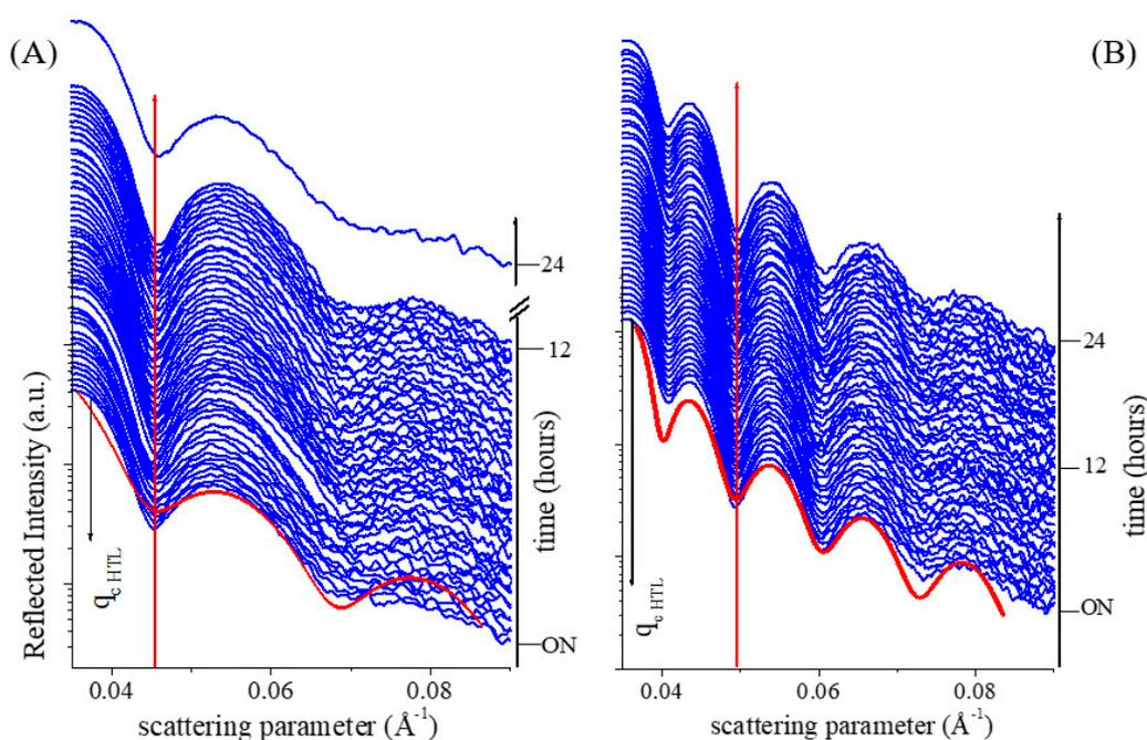
**Figure 2.** In situ time resolved morphological and electron density monitoring glass/HTL samples under illumination, representative of different thicknesses ( $d$ ) taken into account: (A)  $d = 120 \text{ \AA}$ ; (B)  $d = 515 \text{ \AA}$ . Parratt fit (red line)—used to deduce morphological parameters and electron density—is shown for the first pattern.
