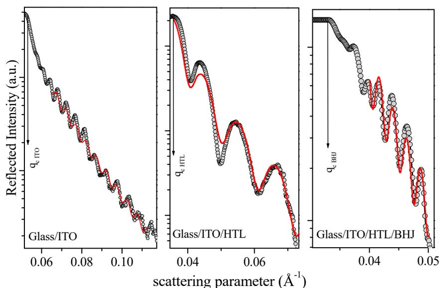
**Figure 1.** Reflectivity edges of the various materials, layer by layer. Red lines are the Parratt fits used to deduce electron density, as follows: glass/ITO,  $\rho_e = 5.6 \times 10^{-5} \text{ \AA}^{-2}$ ; glass/ITO/ K6-P2W18  $\rho_e = 3.04 \times 10^{-5} \text{ \AA}^{-2}$ ; glass/ITO/ K6-P2W18/P3HT:PCBM,  $\rho_e = 1.3 \times 10^{-5} \text{ \AA}^{-2}$ .
