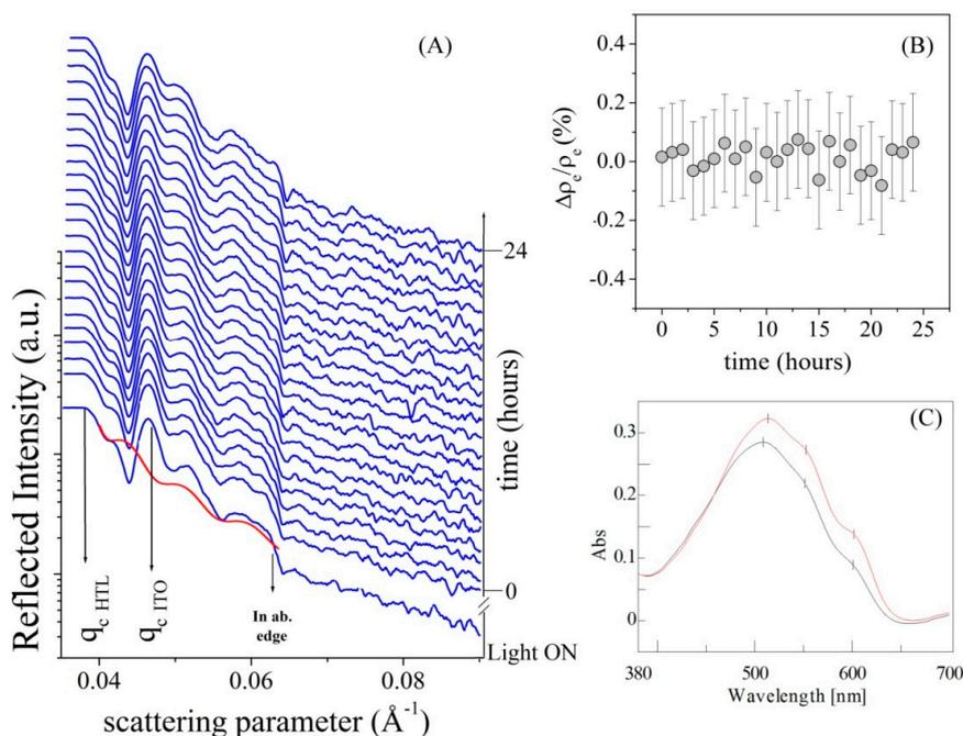
**Figure 3.** (A) In-situ time-resolved EDXR patterns of glass/ITO/HTL collected upon prolonged illumination. As visible, despite the presence of ITO reflectivity and absorption edge, HTL signal is still detected and fitted by Parratt model (red line). (B) Electron density monitoring showing no modification. (C) UV-VIS spectra collected prior (red line) and after illumination (black line).
