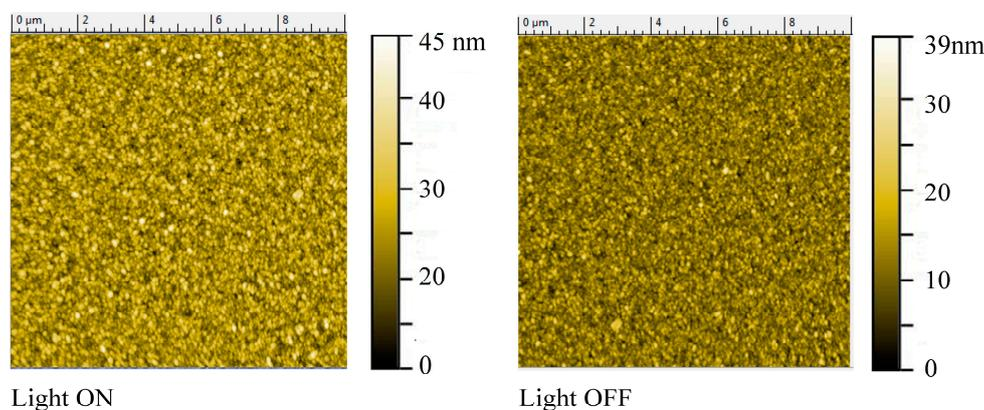
**Figure 4.** AFM images—representative of several investigated portions—collected upon the glass/ITO/HTL intermediate sample shown in Figure 3 ( $d = 520\ \text{\AA}$ ), before and after prolonged illumination, supporting ED-XRR data, proving no morphological modification occurred as a consequence of aging.
