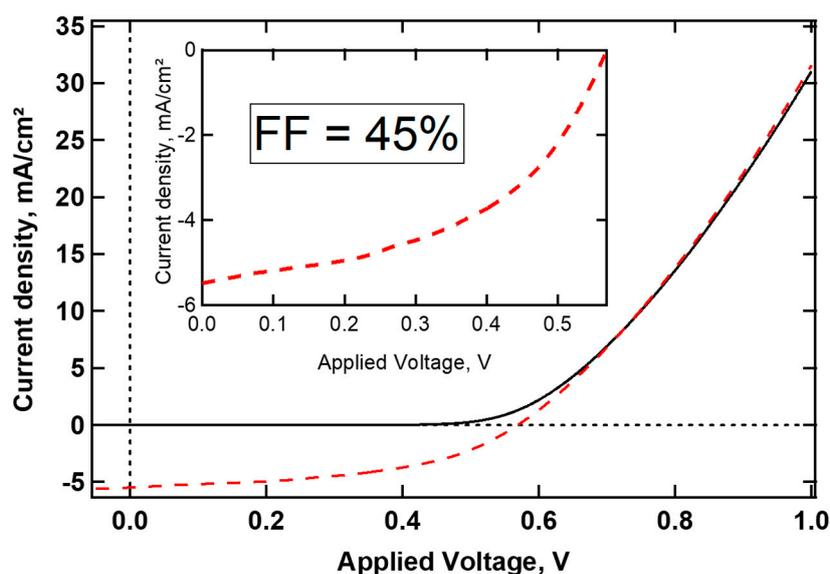
**Figure 6.** Current density as a function of the applied bias of an {ITO/K6-P2W18(>45 nm)/P3HT-PCM (120 nm)/LiF(0.7 nm)/Al} solar cell, at 80 mW/cm<sup>2</sup>. The curve corresponding to the I(V) characterization performed in the dark is reported as a black line; the I(V) curve under illumination is plotted as a red dash line. The inset graph is a zoom into the fourth quadrant to highlight the fill factor, measured at 45%.
