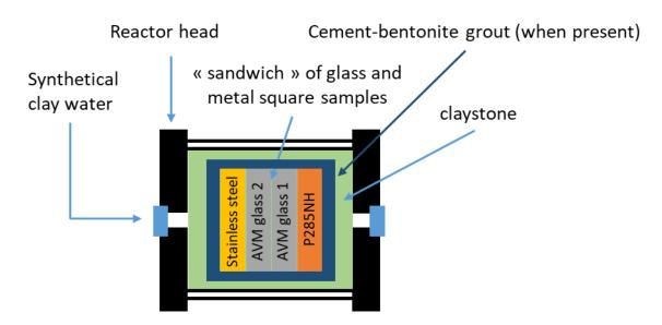
Figure 1: schematic view of the glass/steel/claystone system altered in reactor
