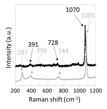
Figure 3:  $\mu$ Raman spectra obtained in the ICP at the AVM glass 1/carbon steel interface without CBG (grey) and with CBG (black) evidencing siderite and chukanovite respectively
