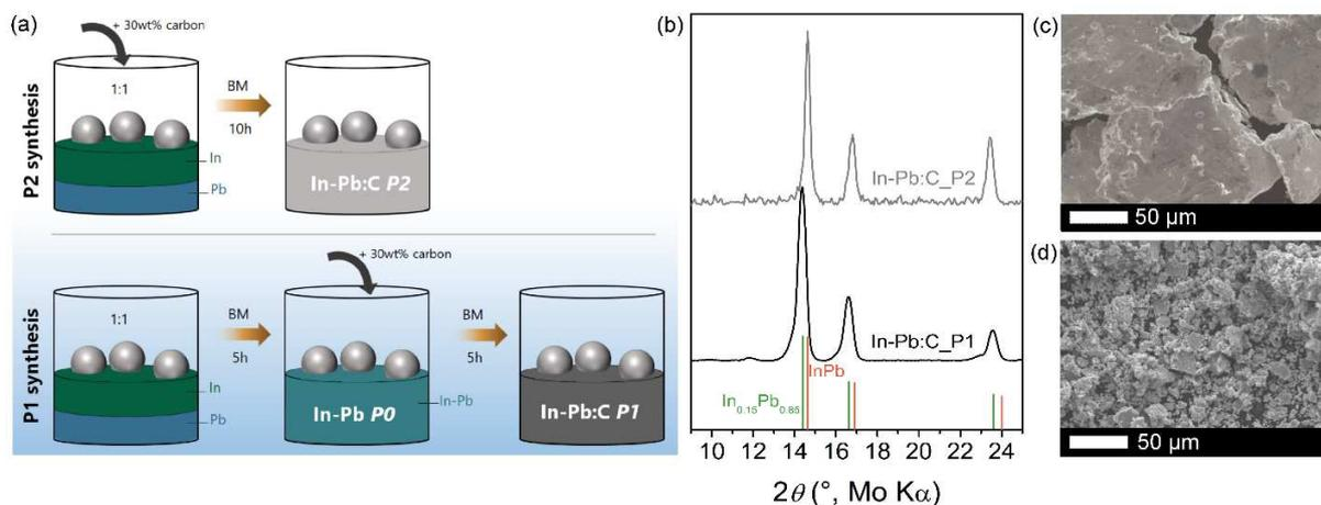
**Fig. 1.** (a) Schematic showing the experimental protocol for the ball-milling (BM) syntheses of P1 and P2 In-Pb:C powders. (b) XRD patterns of the P1 (black) and P2 (gray) In-Pb:C powders with InPb [22] (red) and In<sub>0.15</sub>Pb<sub>0.85</sub> [24] (green) Bragg positions as references. (c, d) Scanning Electron Microscopy (SEM) images of the ball-milled In-Pb P0 and ball-milled composite In-Pb:C P1 powders, respectively.
