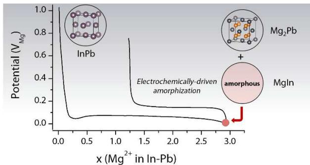
A In-Pb solid solution is investigated as negative electrode for Mg-ion battery and shows reversible alloying with upon magnesiation the formation of crystalline  $Mg_2Pb$  and an electrochemically-driven amorphization of MgIn.
