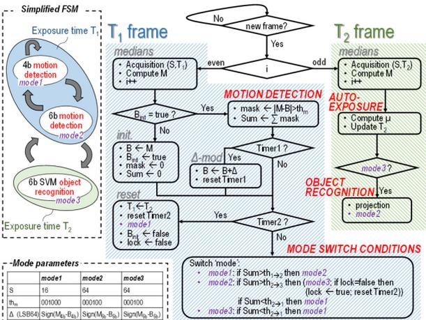
Fig. 3 Algorithm flow chart driven by the on-chip embedded FSM.
