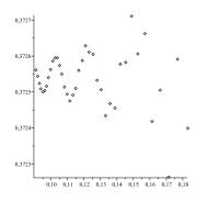
FIG. 11.  $E_{0,k}$ , even-odd averaged, as a function of  $1/k^{2/5}$ . As  $k \to \infty$ , the energy converges—under oscillations—to the point indicated as  $1/k^{2/5} \to 0$ . The plot illustrates the findings of Eqs. (61) and (62).
