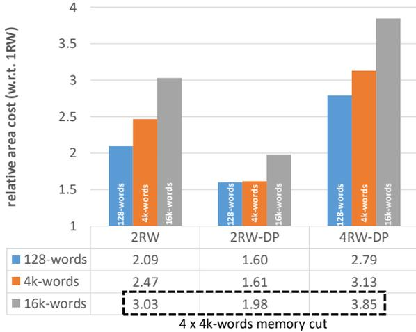
Figure 11 Relative area cost of multi-port memories (*2RW*, *2RW-DP* and *4RW-DP*) to design C-SRAM macro *w.r.t.* a single-port memory (*1RW*) for various sizes (128- to 16k-words).
