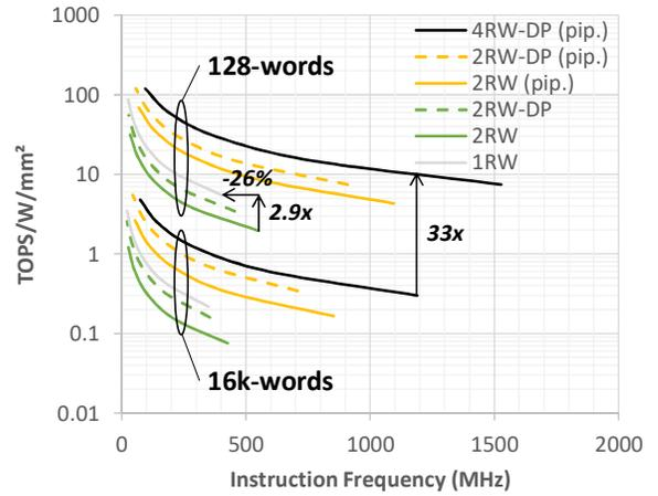
Figure 12 Energy efficiency of vectorized MAC operations per area unit (TOPS/W/mm<sup>2</sup>) performed by a C-SRAM macro according to the instruction frequency for various memory types and sizes (128- and 16k-words).
