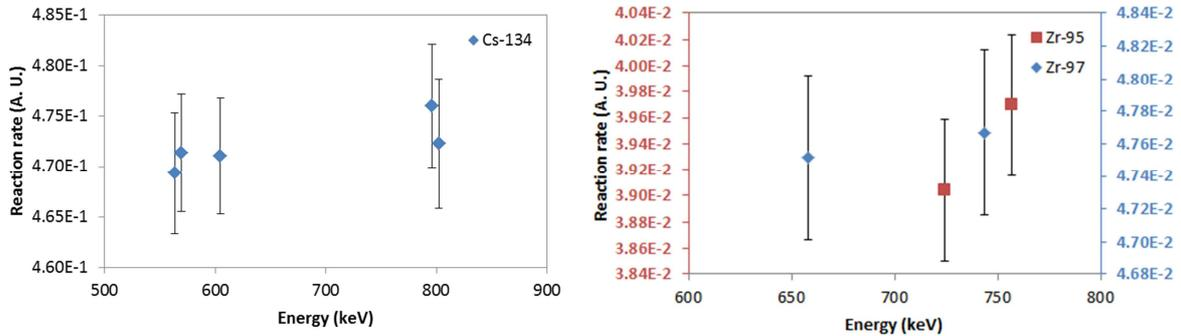
FIG 7: Left: results for  $^{134}\text{Cs}$ . Right: results for  $^{95}\text{Zr}$  (left-hand axis) and  $^{97}\text{Zr}$  (right-hand axis) ( $1\sigma$ ).
