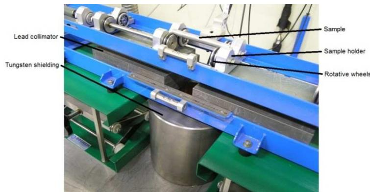
FIG 3: Picture of the gamma spectrometry bench.
