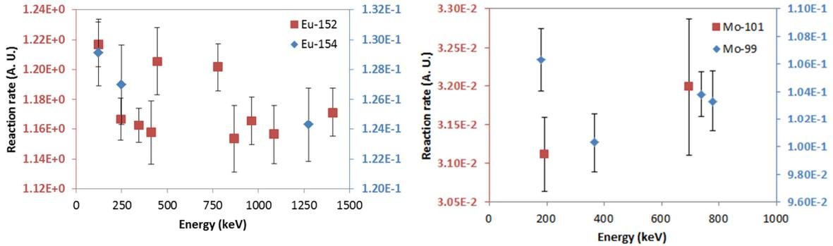
FIG 6: Left: results for  $^{152}\text{Eu}$  (left-hand axis) and  $^{154}\text{Eu}$  (right-hand axis). Right: results for  $^{101}\text{Mo}$  (left-hand axis) and  $^{99}\text{Mo}$  (right-hand axis) ( $1\sigma$ ).
