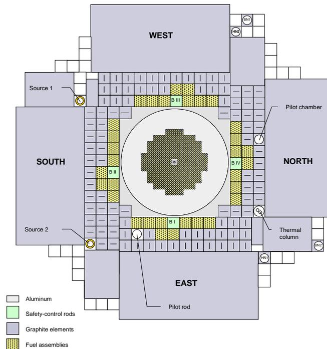
FIG 1: Schematic view of the MINERVE core.
