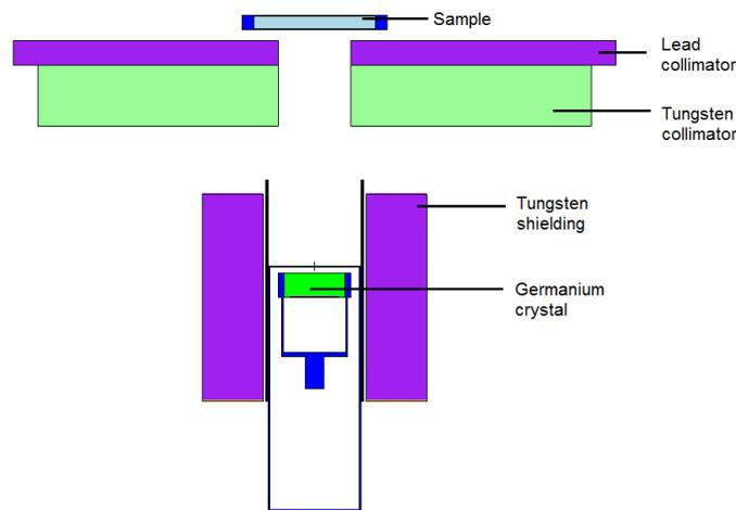
FIG 5: MCNP model of the gamma spectrometry bench with a 10-cm long sample.
