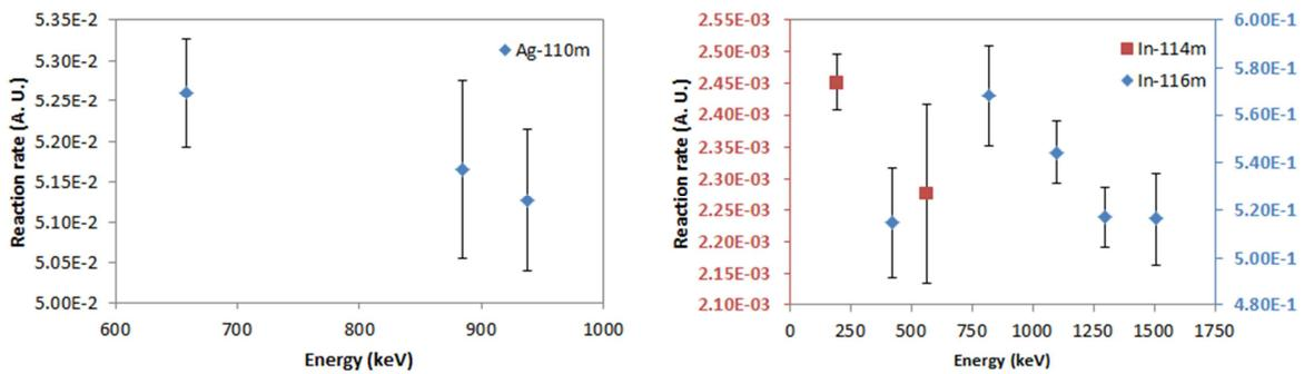
FIG 8: Left: results for  $^{110m}\text{Ag}$ . Right: results for  $^{114m}\text{In}$  (left-hand axis) and  $^{116m}\text{In}$  (right-hand axis) ( $1\sigma$ ).
