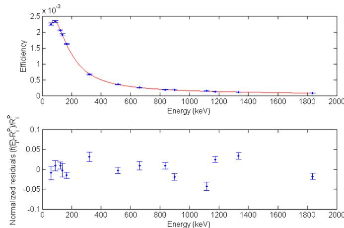
FIG 4: Experimental calibration curve (top) and normalized residuals (bottom).
