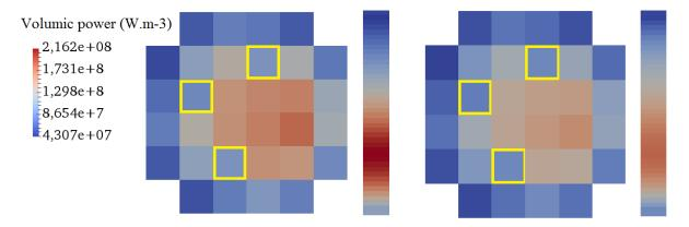
Figure 12. Final power maps of the 2<sup>nd</sup> ejection (left: APOLLO3®, right: CORPUS)
