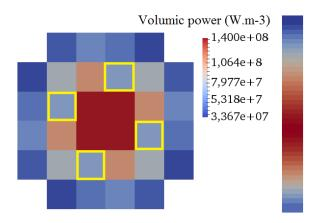
Figure 8. Initial power map of the 2<sup>nd</sup> ejection.
