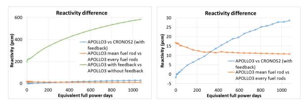
Figure 2. Reactivity differences between the different depletion calculations.
