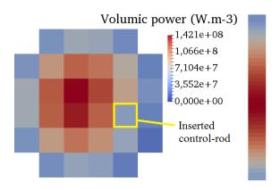
Figure 4. Initial power map of the 1st ejection.
