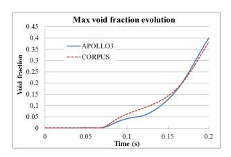
Figure 10. Max void fraction evolutions during 2<sup>nd</sup> ejection.
