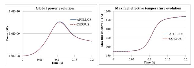
Figure 5. Total power (left) and max fuel effective temperature (right) evolutions during 1st ejection.
