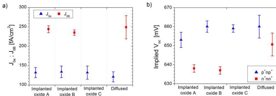
Fig. 3. (a)  $J_{0e}$  and  $J_{0B}$  measured on symmetrical B and P implanted samples respectively and annealed with various oxidation conditions, compared to diffused  $BCl_3$  and  $POCl_3$  samples; (b) Implied  $V_{oc}$  measured after IR firing on the same samples.
