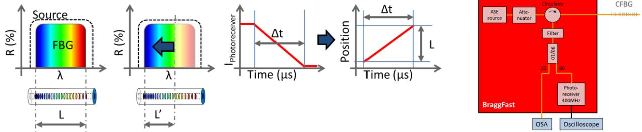
Figure 1. a) Detonation & shock velocity measurement using a CFBG b) the CFBG measurement system.
