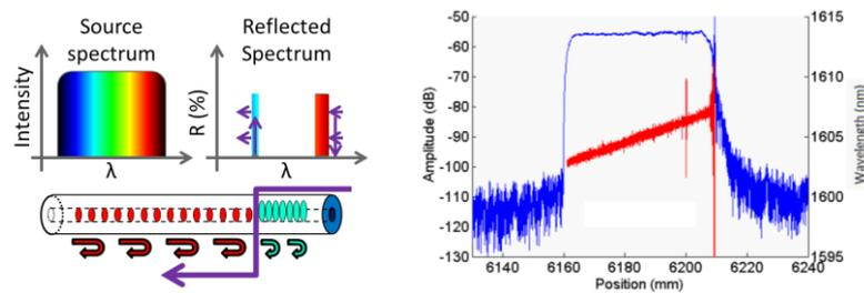
Figure 4. a) High pressure profile measurement using a CFBG. b) type of CFBG: 48-mm long, at 1605 nm & 4-nm wide.
