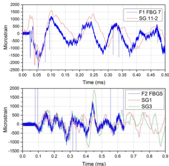
Fig. 4. Electrical strain gauges vs. FBG a) inside the cylinder and near the detonators b) outside the cylinder in the middle of height.
