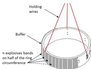
Fig. 2. Sketch of an experimental setup in the case of a ring sample.
