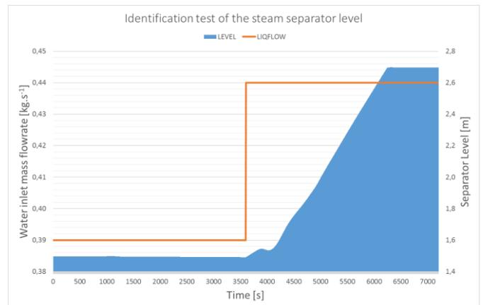
Fig. 6. Steam separator level identification test
