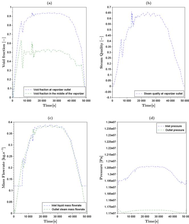
Fig. 5. Excerpts of the fluid thermal-hydraulic properties available from the co-simulation results (time evolutions over one day).
