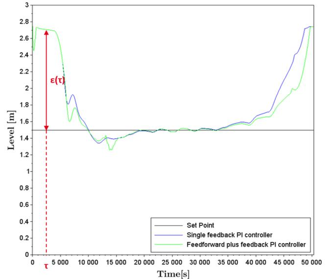
Fig. 7. Comparison of the two control strategies during an ideal sunny day with clear sky (no cloud passage)
