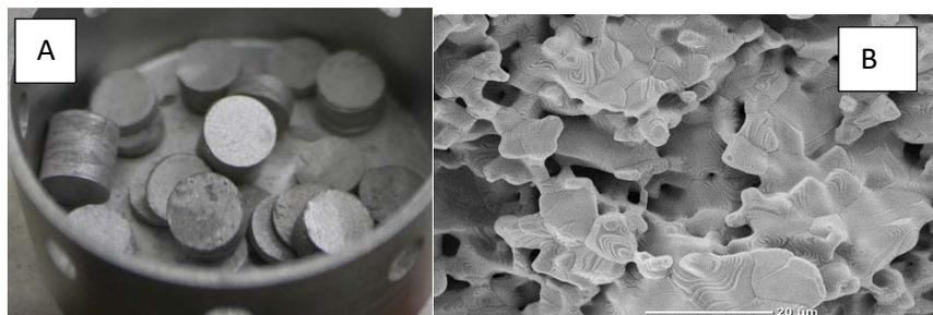
Figure 8: A) synthesized pellets (diameter about 8 mm) after carbo-reduction cycle and B) surface micrograph observed by SEM
