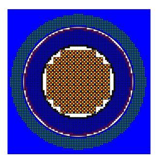
Figure 2: X-Y representation of the TRIPOLI4® modelling of the Fast/Thermal optimized configuration Blue: light water – Green:  $UO_2$  3.7% enrichment – Purple: Metallic U 30% enrichment Navy: natural  $UO_2$  – Black:  $B_4C$  absorber – White: Air The central cells are the one presented in Fig.1
