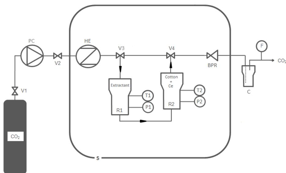
**Fig. 3.** Experimental setup used to measure the solubility of amidophosphonate ligands in supercritical  $\text{CO}_2$ . V1, V2, V3 and V4, valves; PC,  $\text{CO}_2$  pump; HE, heat exchanger; R1, solubilization reactor; R2, extraction reactor; BPR, back-pressure regulator; S, stove; C, collector; F, mass flow meter.
